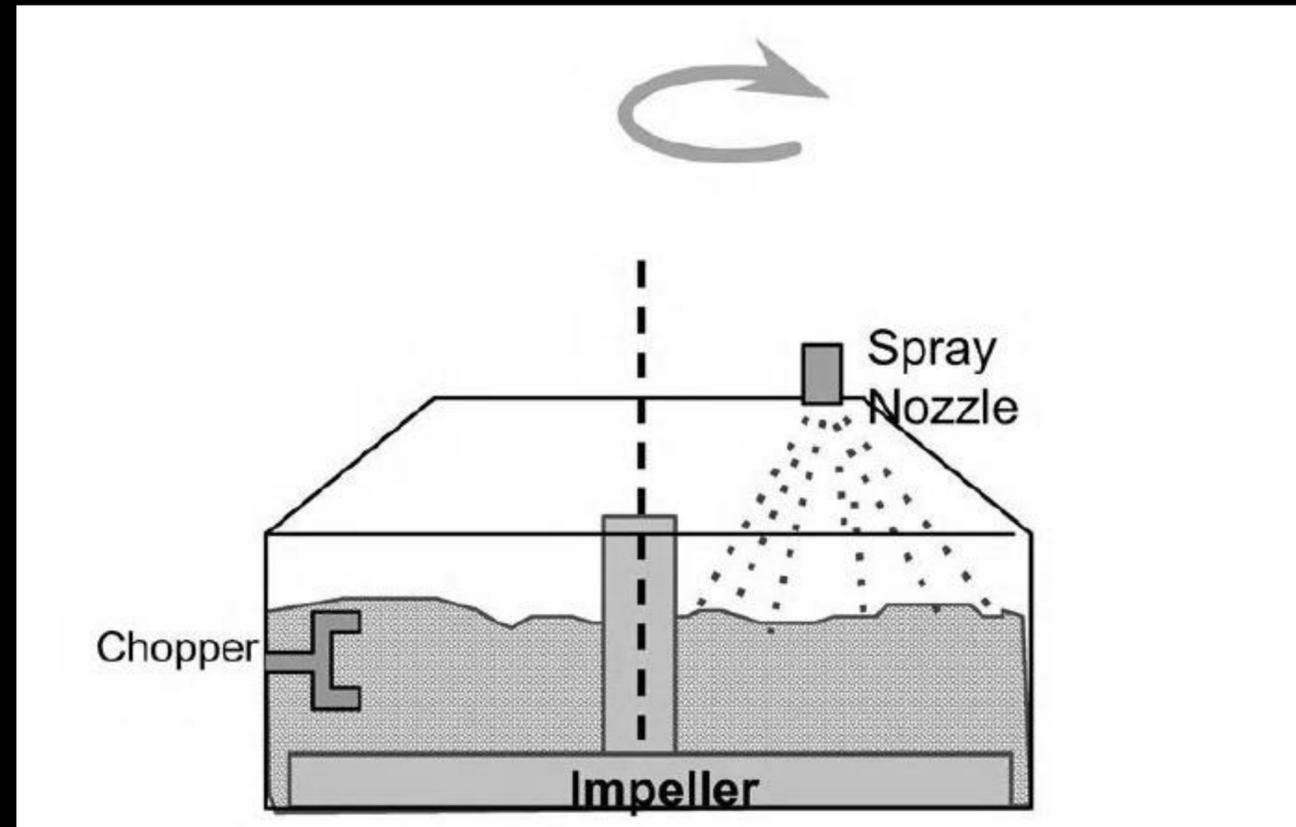
**It consists of agglomerating one or different powders by spraying a liquid binder over the bed of powders under a vigorous mixing.**
